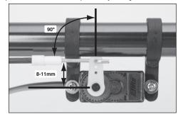
After installing the tail rotor pushrod linkage on the tail servo arm, and ensuring the tail servo is still centered electronically, adjust the length of the pushrod so the tail pitch slider is centered on the tail rotor shaft, between the tail case and tail hub.
